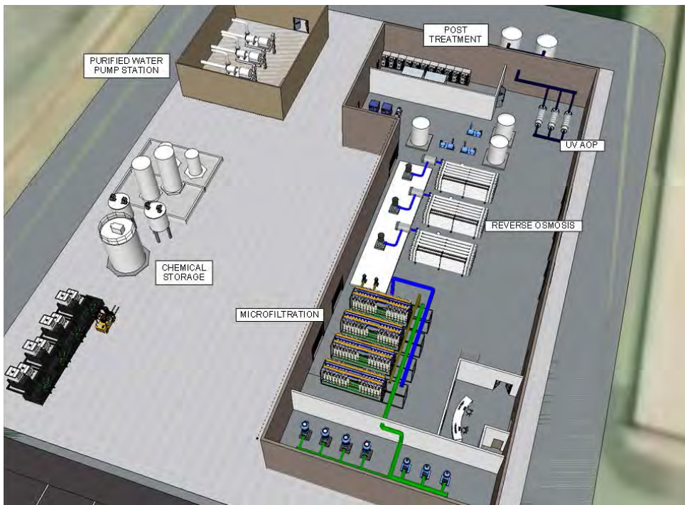
Figure 7.17 Livermore FAT AWPf Layout (Side View)
