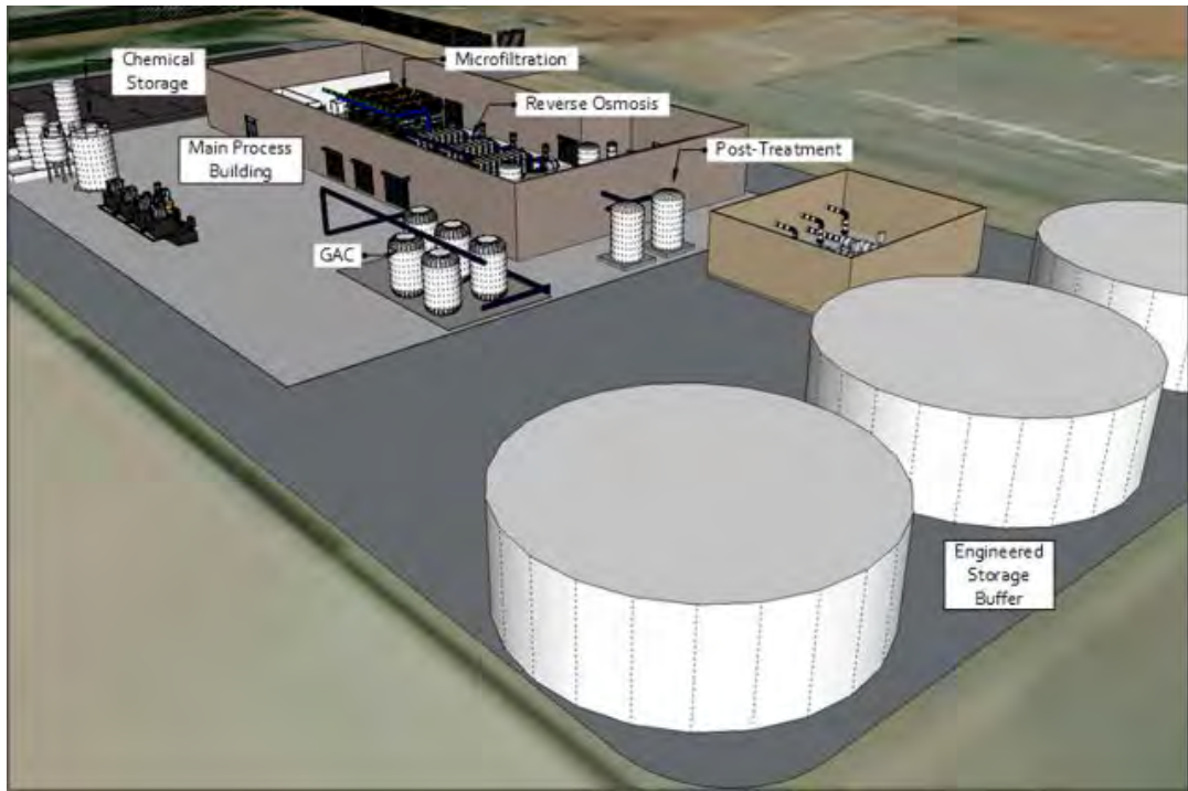
Figure 7.14 Livermore AWPf Layout (Iso View)
