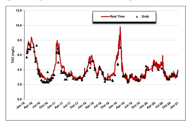
Figure 3-17. Comparison of Banks Real-time and Grab Sample TOC Data, 1:1 Graph, 2016 to 2020
