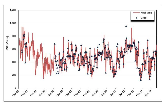
Figure 4-47. Comparison of O'Neill Forebay Outlet Real-time and Grab Sample EC Levels, 1:1 Graph, 2011 to 2020
