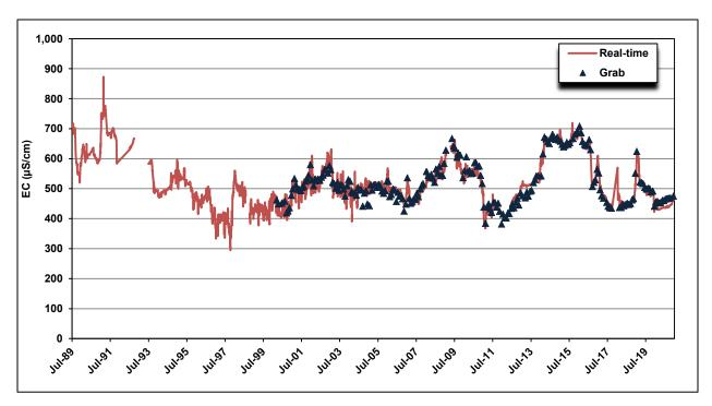
Figure 4-38. Comparison of Pacheco Real-time and Grab Sample EC Data, 1:1 Graph, 2000 to 2020
