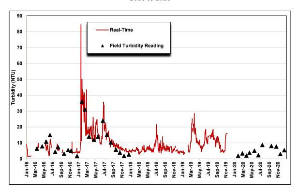
Figure 8-49. Comparison of Check 41 Real-time and Field Sample Turbidity Data, 2016 to 2020, 1:1 Graph
