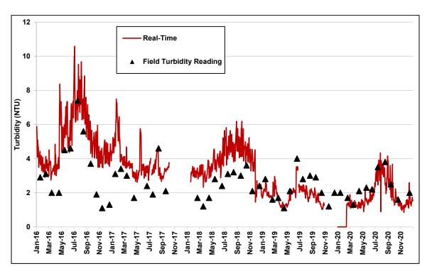
Figure 8-34. Comparison of Pacheco Real-time and Field Sample Turbidity Data, 2016 to 2020, 1:1 Graph
