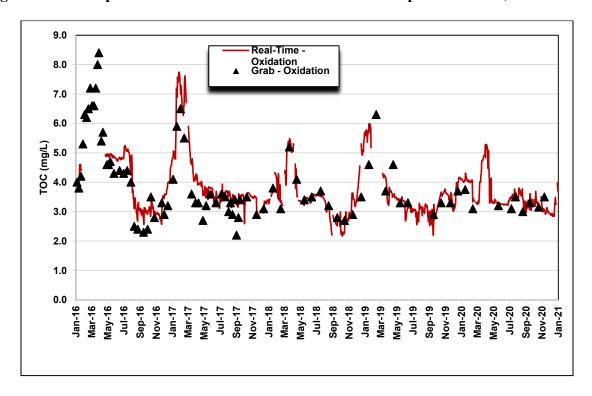
Figure 3-41. Comparison of Gianelli Real-time and Grab Sample TOC Data, 2016 to 2020, 1:1 Graph
