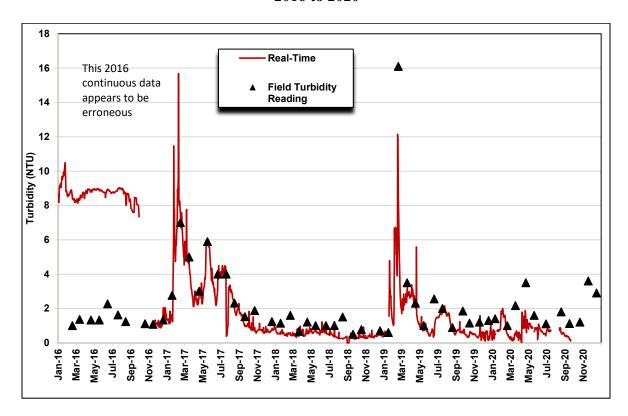
Figure 8-57. Comparison of Devil Canyon Real-time and Field Sample Turbidity Data, 2016 to 2020, 1:1 Graph
