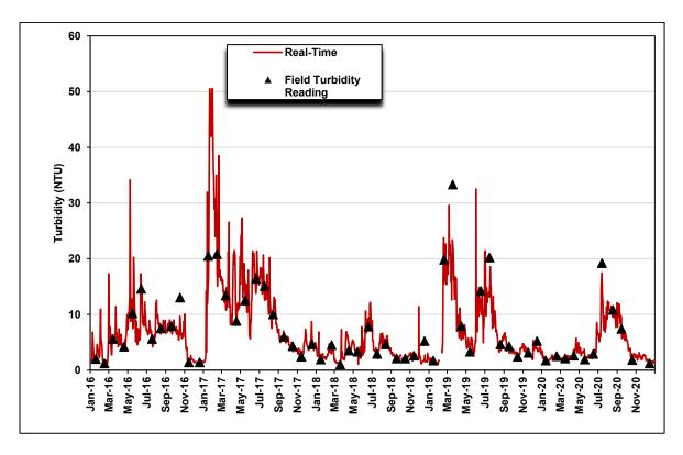
Figure 8-45. Comparison of Check 21 Real-time and Field Sample Turbidity Data, 2016 to 2020, 1:1 Graph
