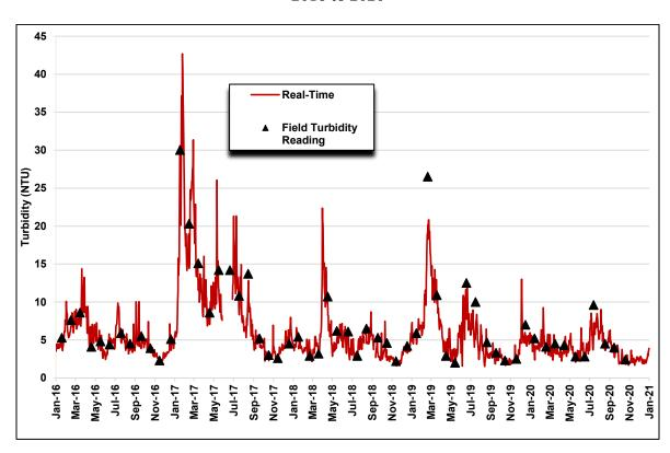
Figure 8-41. Comparison of Check 13 Real-time and Field Sample Turbidity Data, 2016 to 2020, 1:1 Graph
