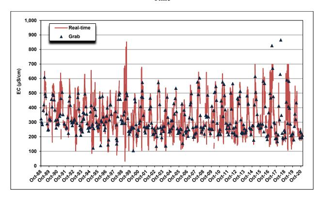
Figure 4-21. Comparison of Barker Slough Real-time and Grab Sample EC Data, 1:1 Graph, 2011 to 2020
