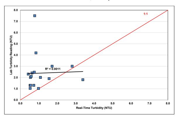
Figure 8-54. Comparison of Castaic Outlet Real-time and Field Sample Turbidity Data, 2016 to 2020, 1:1 Graph
