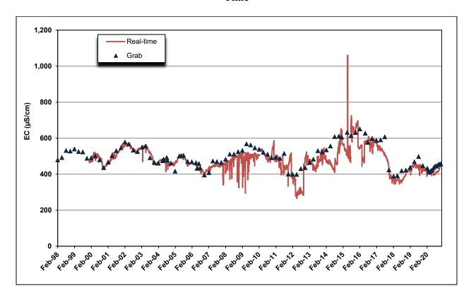
Figure 4-62. Comparison of Castaic Outlet Real-time and Grab Sample EC Levels, 1:1 Graph, 2011 to 2020
