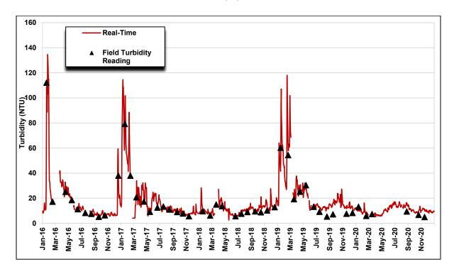
Figure 8-19. Comparison of Barker Slough Real-time and Field Turbidity 2016 to 2020 Data, 1:1 Graph
