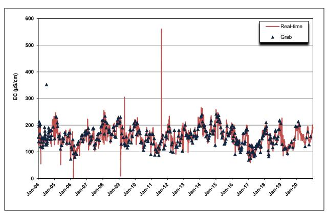
Figure 4-6. Comparison of Hood Real-time and Grab Sample EC Data, 1:1 Graph, 2011 to 2020
