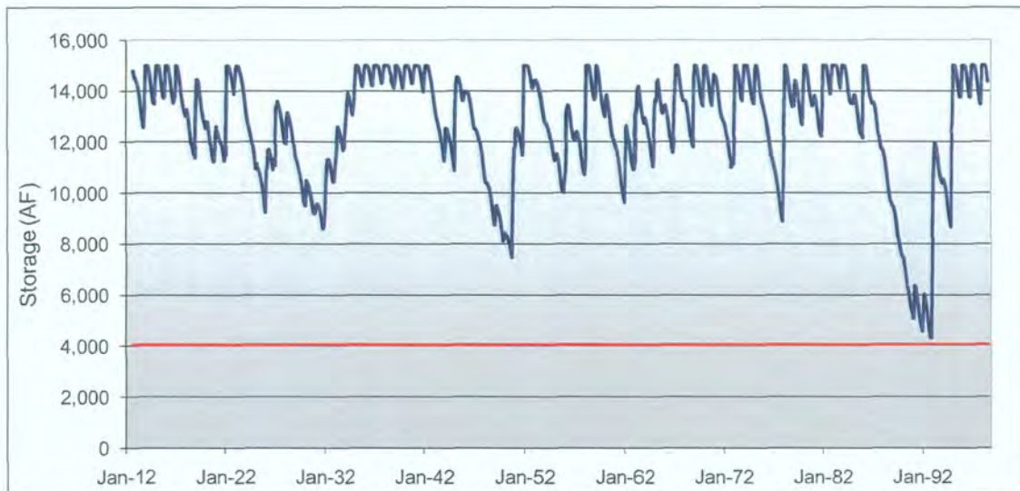
Figure 4-6 Storage Volume Time History of Proposed Arroyo Mocho Reservoir Under Long Term Yield Withdrawal
