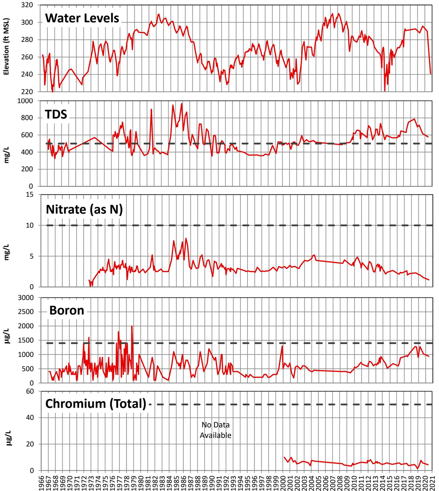
Well Depth = 575'; Wellhead Elevation = 344'; Well Screen Depth: 250 to 570' bgs. Minimum Threshold = - - - - -
