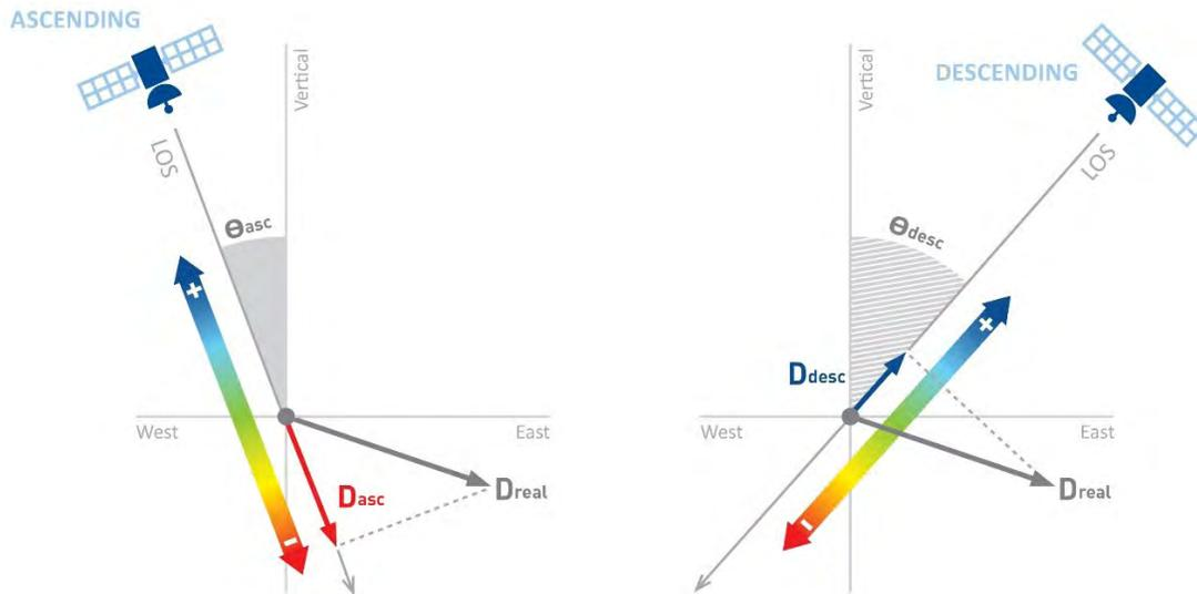
Figure 4: SqueeSAR measures the projection of real movement ( $D_{real}$ ) onto the LOS. The same real movement ( $D_{real}$ ) will produce a different value from a different LOS (different inclination or different acquisition geometry).
