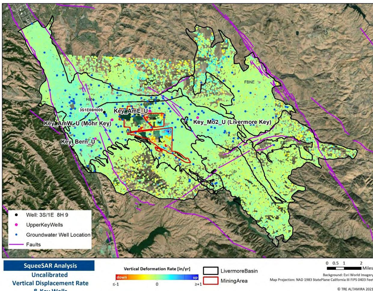
Figure 12: Key well locations, ground displacement and faults.
