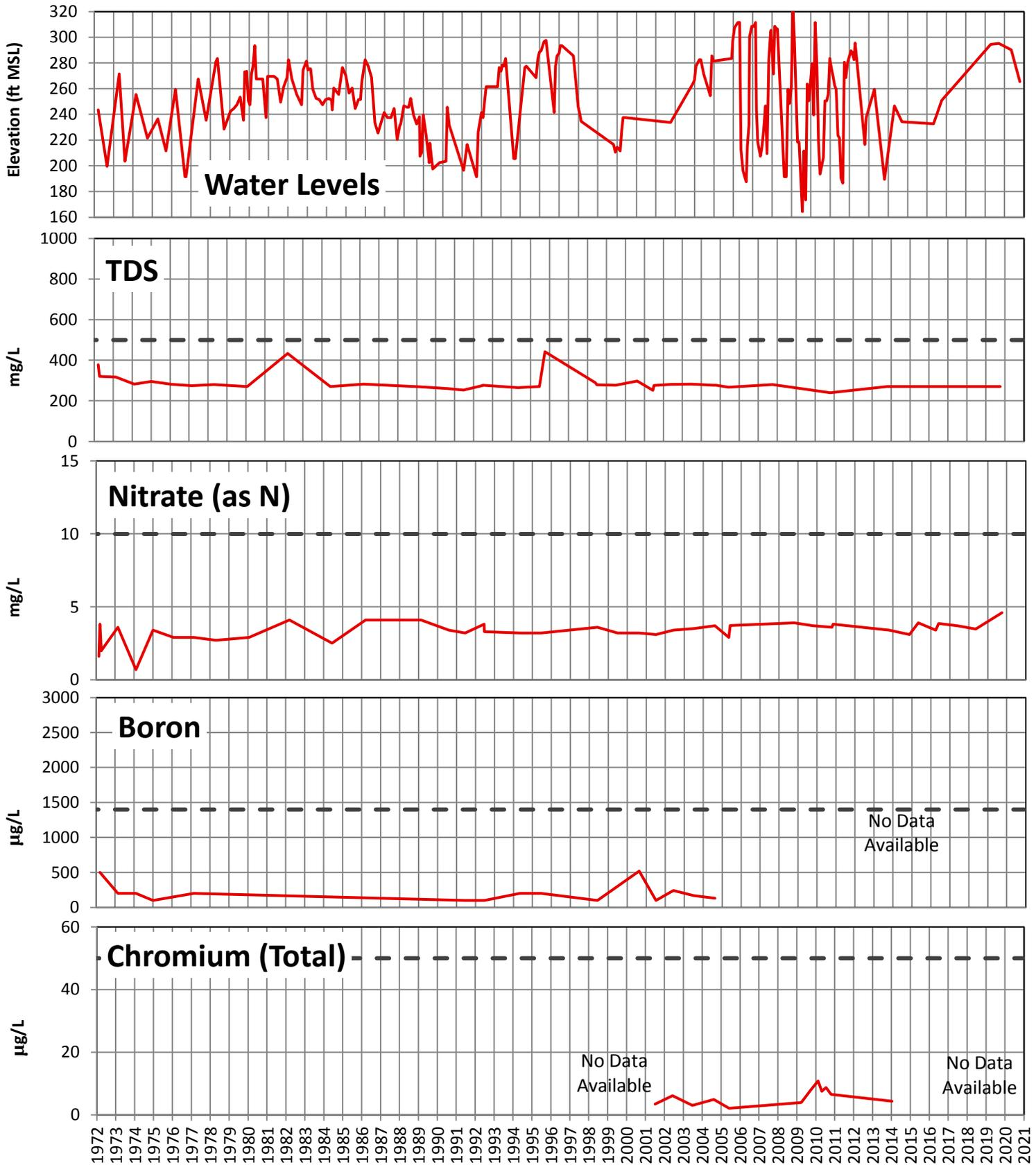
Well Depth = 510'; Wellhead Elevation = 429'; Well Screen Depth: 300 to 490' bgs.
