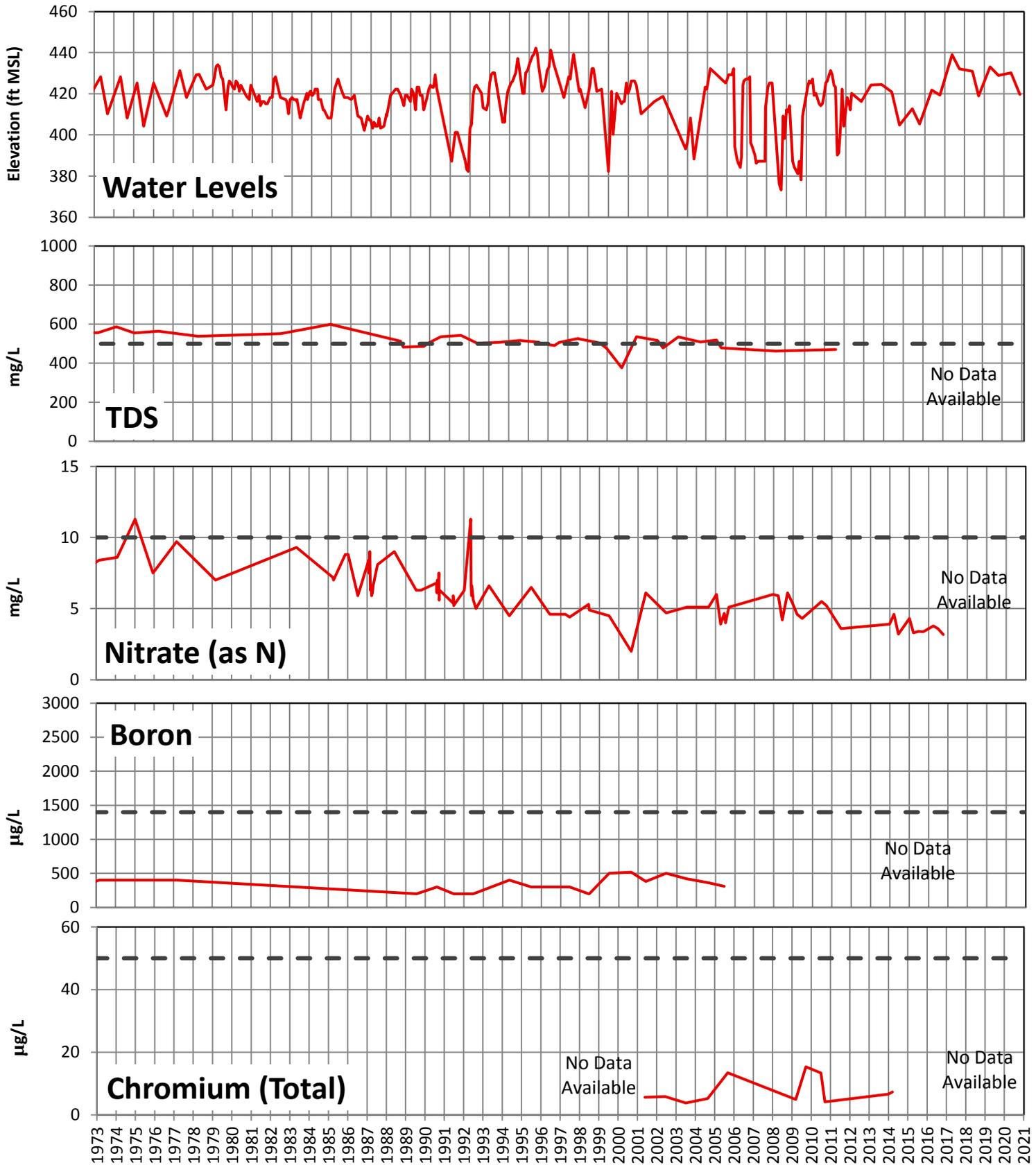
Well Depth = 273'; Wellhead Elevation = 466'; Well Screen Depth: 122 to 263' bgs. Minimum Threshold =
