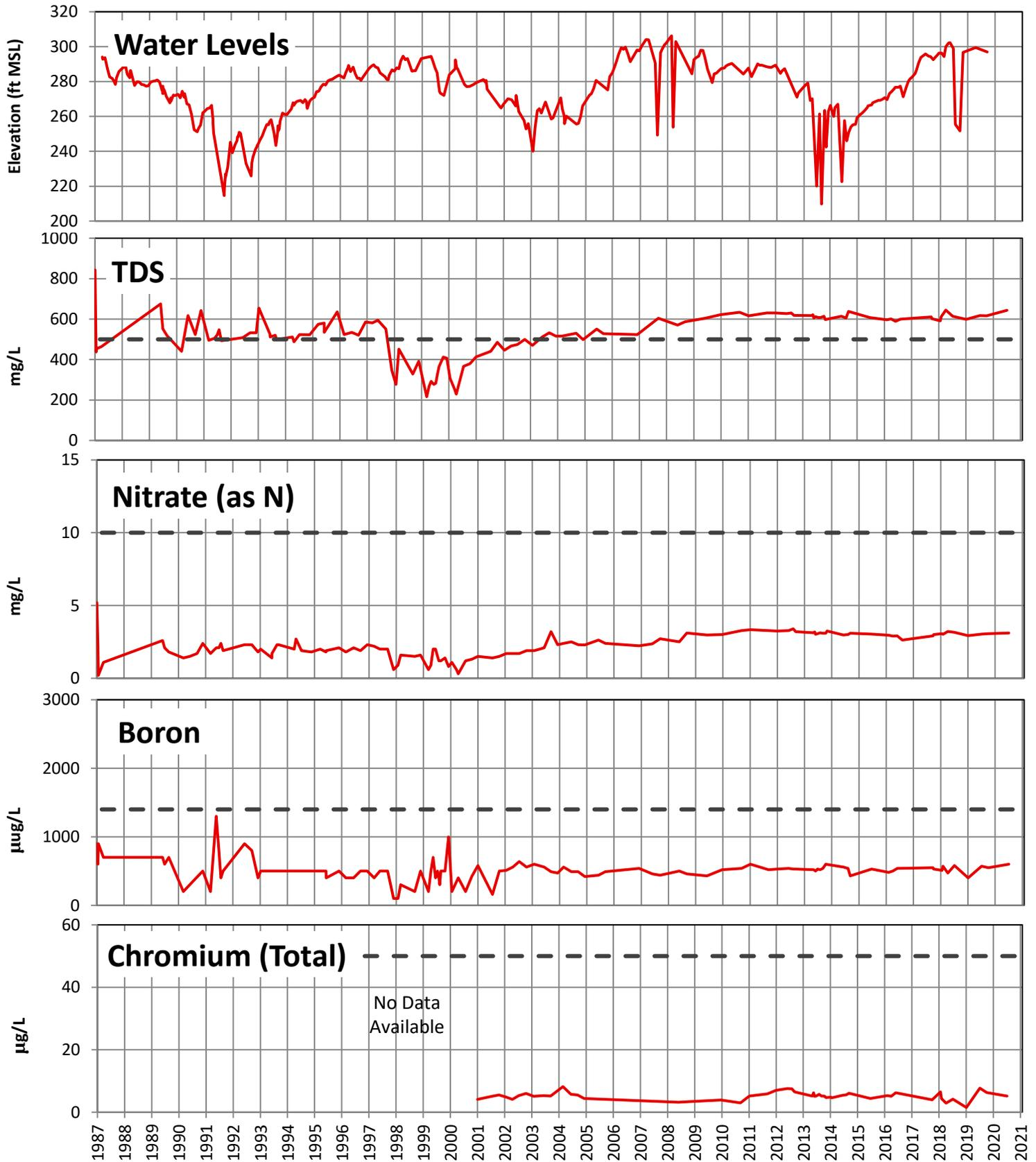
Well Depth = 500'; Wellhead Elevation = 327'; Well Screen Depth: 215 to 490' bgs. Minimum Threshold = - - - - -
