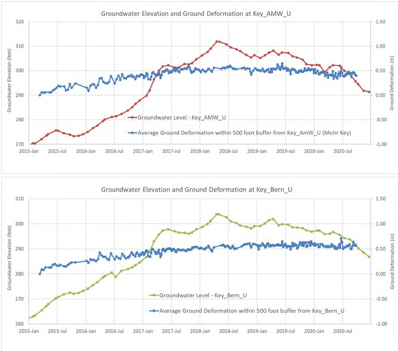
Figure 14: Groundwater elevation vs. ground displacement at Key\_AMW\_U (top) and Key\_Bern\_U (bottom).
