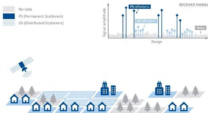
Figure 3: Schematic of PS and DS radar targets.
