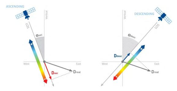
Figure 4: SqueeSAR measures the projection of real movement (D<sub>real</sub>) onto the LOS. The same real movement (D<sub>real</sub>) will produce a different value from a different LOS (different inclination or different acquisition geometry).
