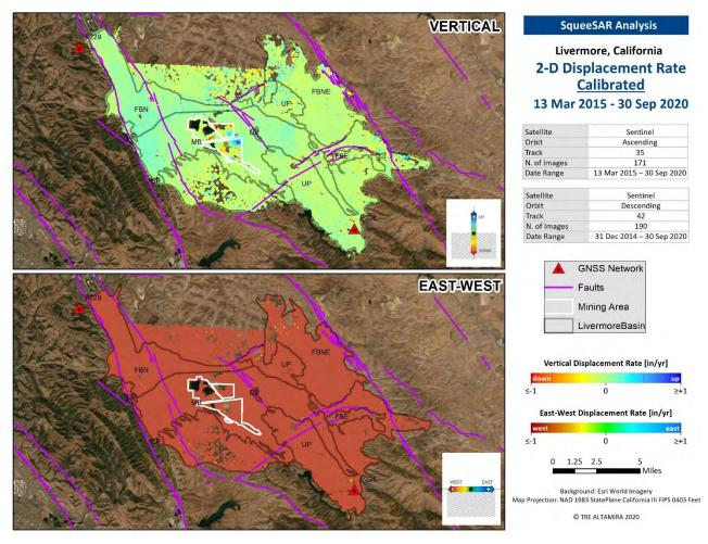
Figure 8: East-West and Vertical calibrated displacement rates over the AOI for the entire study period.
