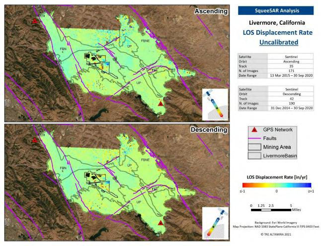
Figure 7: Ascending and Descending uncalibrated displacement rates over the AOI for the entire study period.
