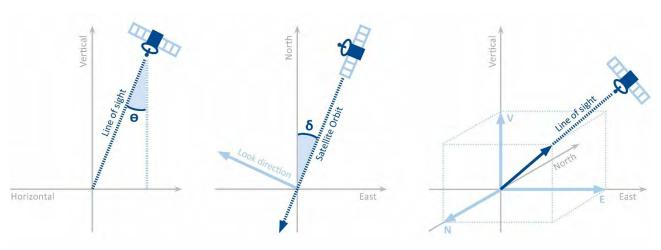
Figure 17: Geometry of the image acquisitions along the descending orbit.
