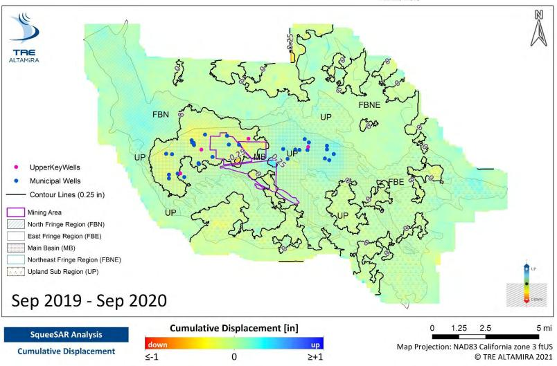
Figure 11: Interpolated map showing annual (September to September) ground displacement from 2019 to 2020. Contour lines have a 0.25-inch interval.
