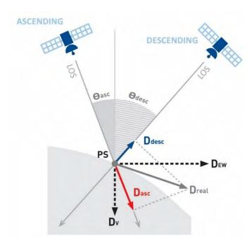
Figure 5: Example of motion decomposition combining ascending and descending acquisitions geometry.
