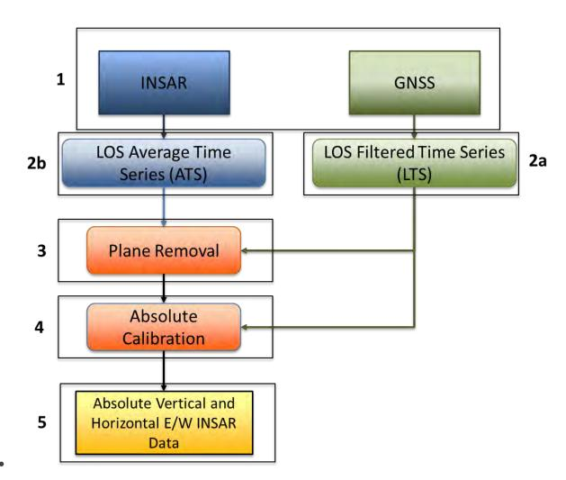
Figure 18: Diagram of the calibration methodology applied over the site.
