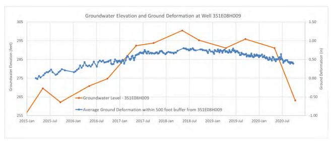
Figure 15: Groundwater elevation vs. ground displacement at well 3S1E08H009.
