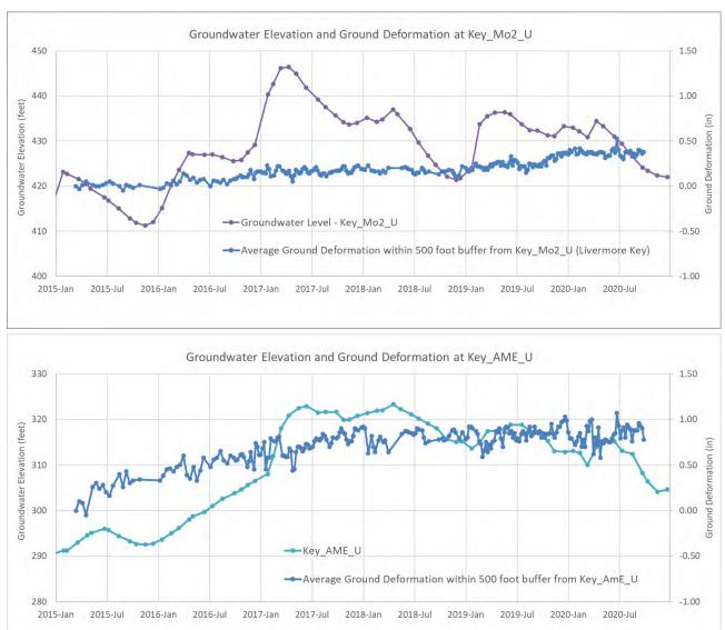
Figure 13: Groundwater elevation vs. ground displacement at Key\_Mo2\_U (top) and Key\_AME\_U (bottom).
