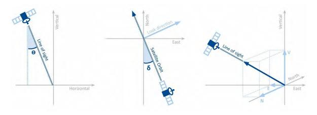
Figure 16: Geometry of the image acquisitions along the ascending orbit.
