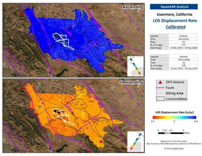
Figure 6: Ascending and Descending calibrated displacement rates over the AOI for the entire study period.
