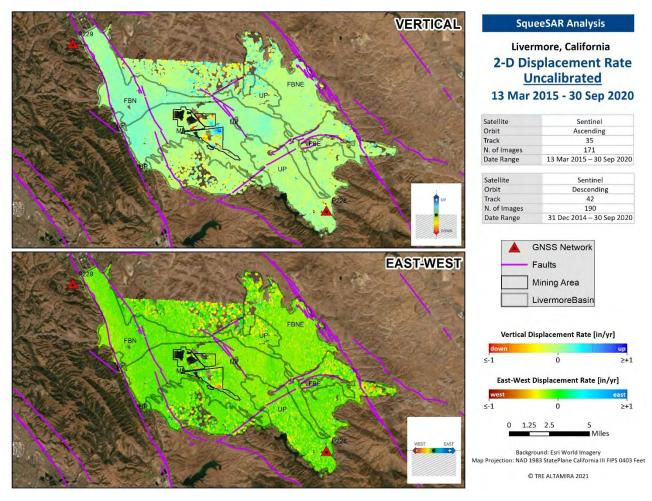
Figure 9: East-West and Vertical uncalibrated displacement rates over the AOI for the entire study period.
