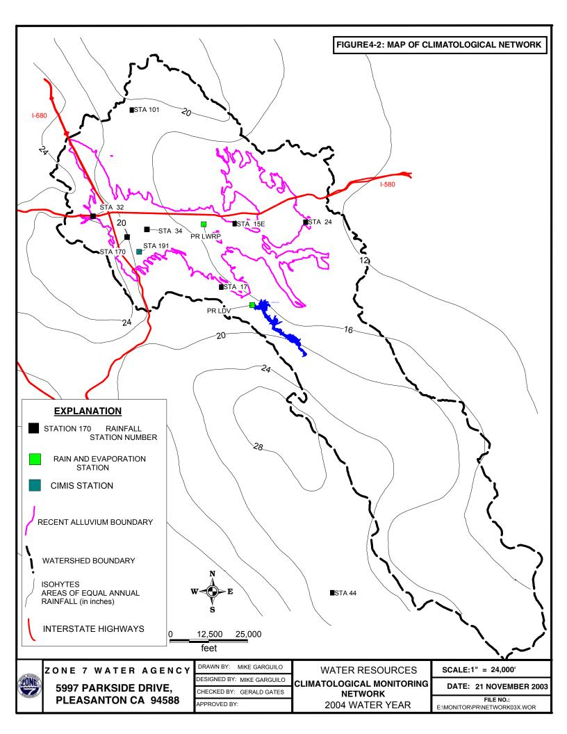
The program also includes two evaporation stations that collect data with an evaporation pan. The Lake Del Valle (LDV) station, operated by DWR is a part of LDV operations. The Livermore Water Reclamation Plant (LWRP) operates the LWRP station as part of their wastewater treatment plant operations.
