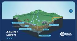
We draw from the groundwater basin using our well system to pump water out when imported surface water supplies are limited. This type of groundwater management will continue to keep our groundwater basin healthy and sustainable and maintains water reliability for our community even in times of drought.
